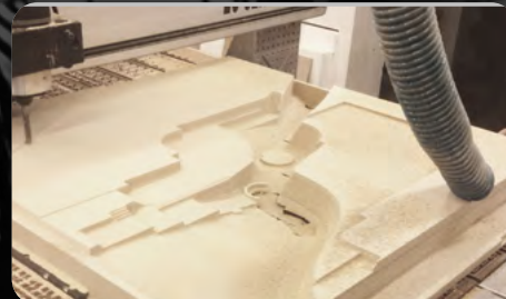
1_CNC BASE AND LASER CUT WALLS
